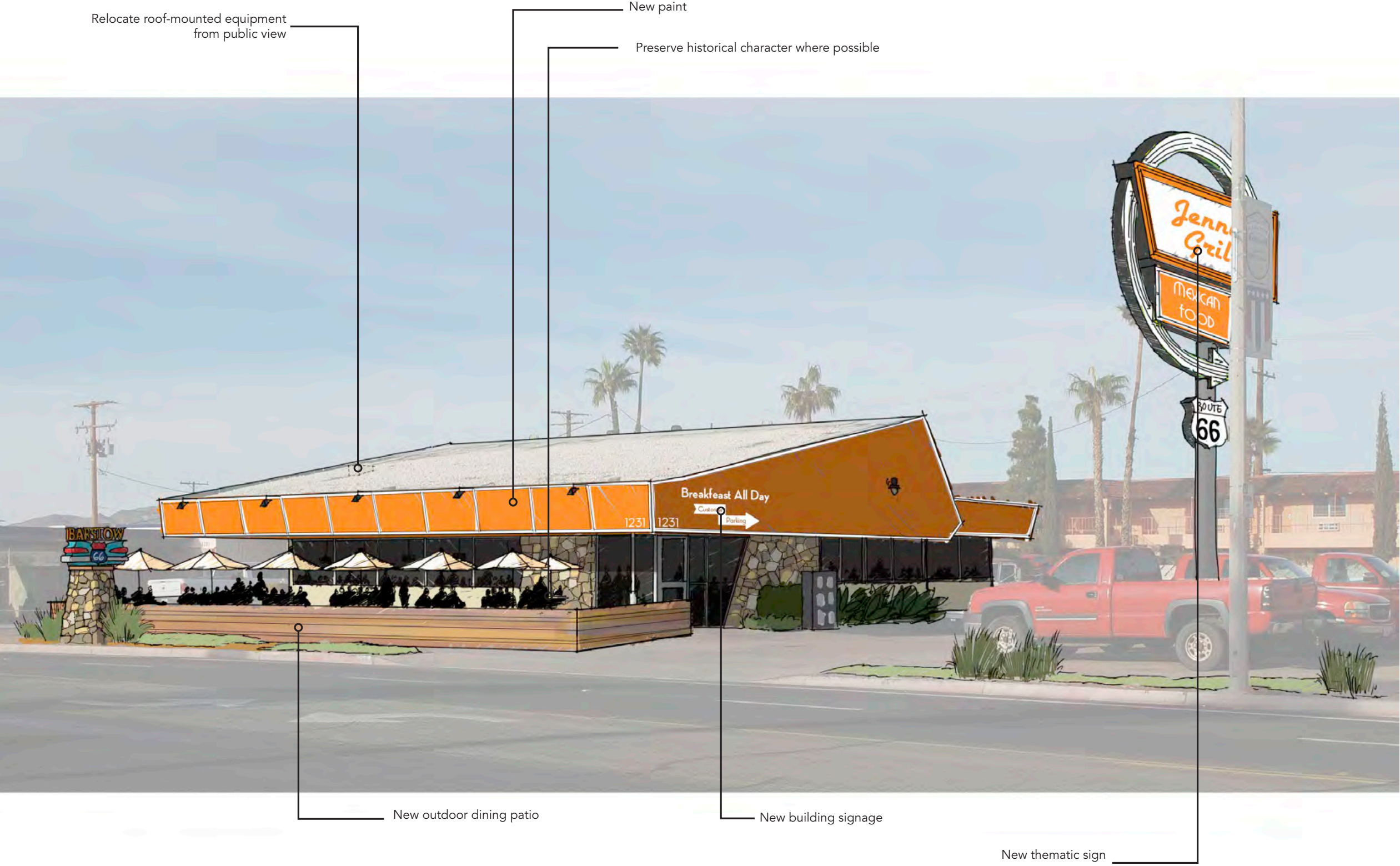
Figure 4.13 LEVEL 3 FAÇADE IMPROVEMENTS
