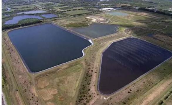
**Description:** Pond #3 has not been drained or maintained since 2013 due to inability to pump from pond #4. With the upgrades to the east irrigation station, staff will drain, remove any solids, rip the bottom, and rehab the banks of the pond.
