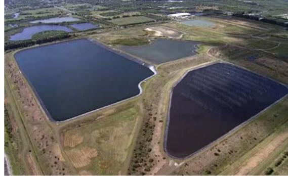
**Description:** Pond #4 has not been maintained since it was drained in 2013 due to large amount of debris found in the bottom of it. With the upgrades to the east irrigation station, staff will remove the large amount of solids, rip the bottom, finish the installation of piping, and pump repairs needed to get the pond back into operation.
